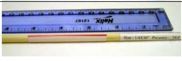
\*The exact sizes of the dowel and straw may vary. The important thing is to match the straw and dowel diameters so that the straw slides easily along the dowel.
